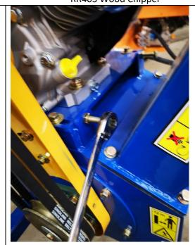
After adjustment, you can see the engine plate is now pushed away from the adjustment bolt-the tension on the belt has been increased
