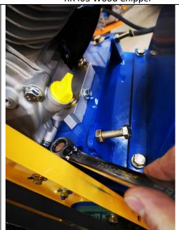
Now that the engine mounting bolts are loose, we can loosen off the jam nuts on the two belt adjustment bolts
